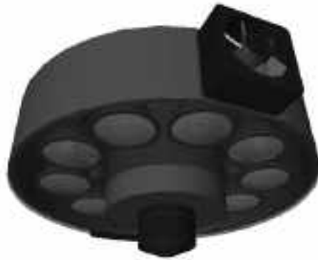
Figure 1-3: Camera with 10 halogen lamps and infrared filter mounted in a round box
