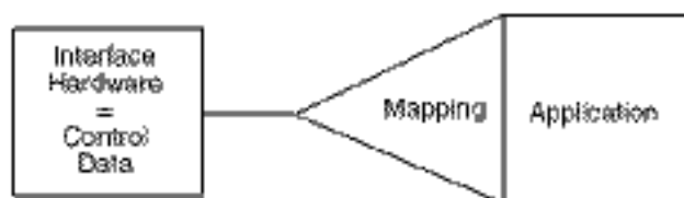
Figure 2.2: Standard system architecture with external interface hardware
