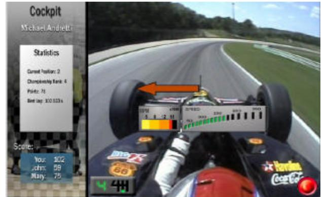
**Figure 6:** Animated overlay based on streamed telemetry data.
