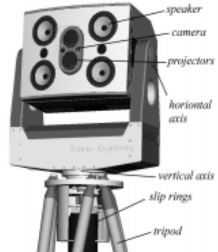
Figure 1: The EVE stereo-projection device features two rotational degrees of freedom, two video projectors (with polarized lenses), a stereo audio system and a built-in infrared camera for tracking purposes
